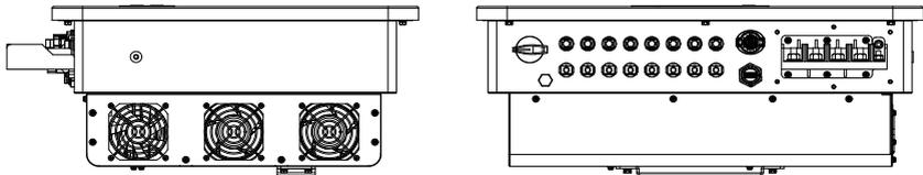
Figure 2-4 Bottom view (take 25KW for example)
