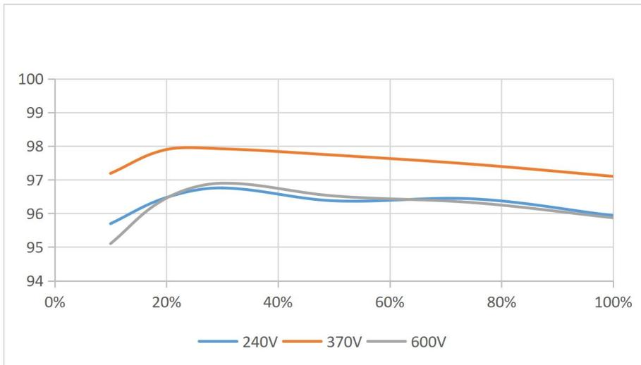
Figure 2-9 Power efficiency curve (take 25KW for example)
