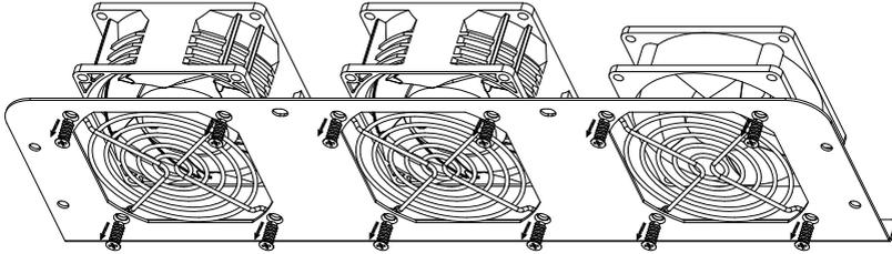
Figure 7-2 remove the fan and protective cover
