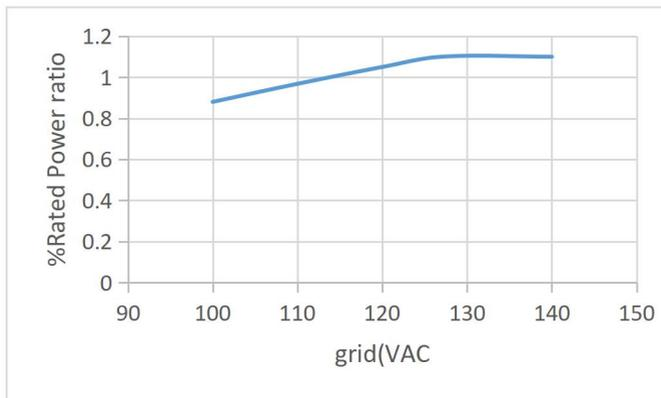
Figure 2-10 Rated Power ratio vs Grid Voltage
