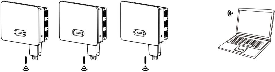
Figure 4-21 Connect multiple USB acquisition stick (WIFI version) to wireless router
