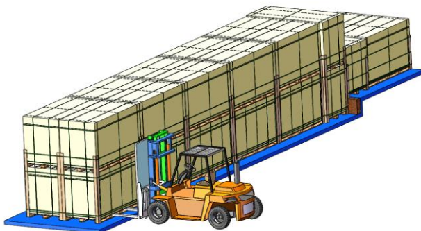
Vertical portrait package unloading with forklift
