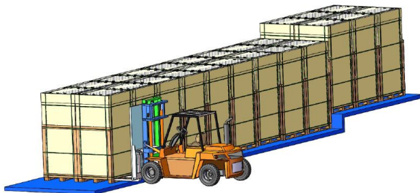
Vertical portrait package unloading with forklift
