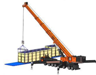
Vertical portrait package unloading with crane
