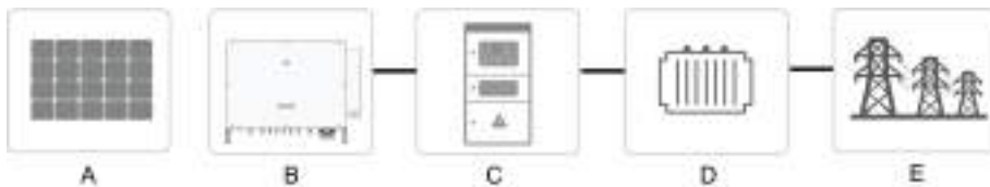
figure 2-1 Inverter Application in PV Power System
